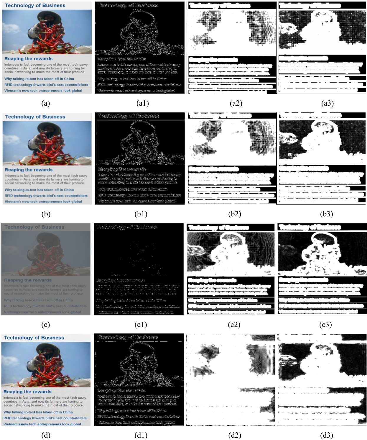
FIGURE 2. A illustration edge features in Gradient domain of SCIs: [Column 1]: (a) a reference SCI. (b) SCI with Gaussian blur (c) SCI with contrast change. (d) SCI with JPEG2000 compression [Column 2] their Gradient Profile Sharpness (GPS) [Column3 and 4] their Edge Brightness and contrast features in gradient domain respectively.
