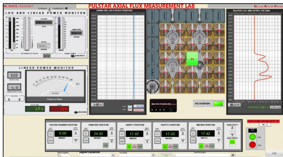
Fig. 7. Axial Flux Measurement Laboratory GUI; note the position of the dry well highlighted in green in fuel assembly D4, and the detector current trace at right.
