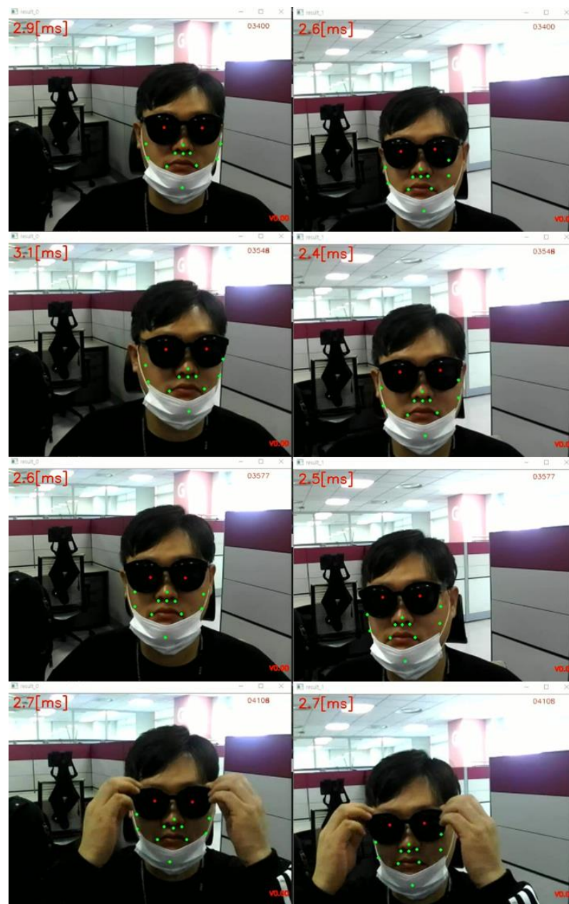
Figure 6. Seamless eye tracking for a user wearing sunglasses. A stereo RGB camera was used for 3D position conversion. The two columns show the left and right images from the stereo camera.
