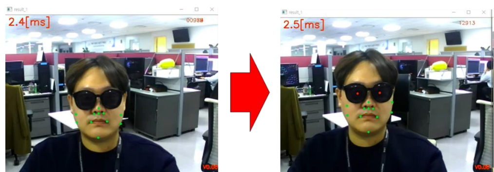
Figure 5. Eye position estimation by a supervised linear regression algorithm. Nonoccluded area shape tracking points ( left, green dots ), with eye positions inferred using these points ( right, red dots ).
