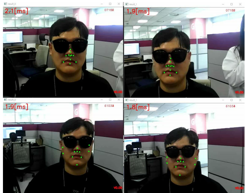
Figure 4. Nonoccluded area shape point candidates identified by a greedy search algorithm: nose–mouth points ( 1st row ) and nose–mouth–face boundary points ( 2nd row ). Each column shows the left and right images from the stereo camera.
