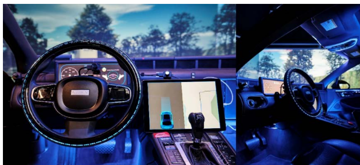
Fig. 2: Integration and composition of HMI elements in driving simulator
