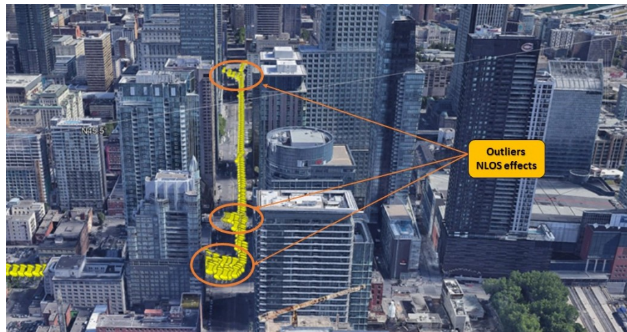
Figure 35. GNSS signals data collection in a Montreal urban environment with high buildings as obstacles.
