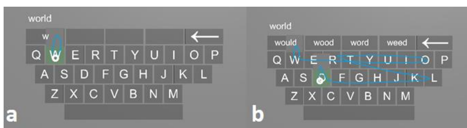
Figure 3-3. An example of typing the letter 'w' (a) and the word 'world' (b) in the Head approach.
