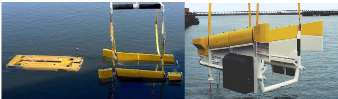
Figure 14. MODUS docking station, source: [Modus].
