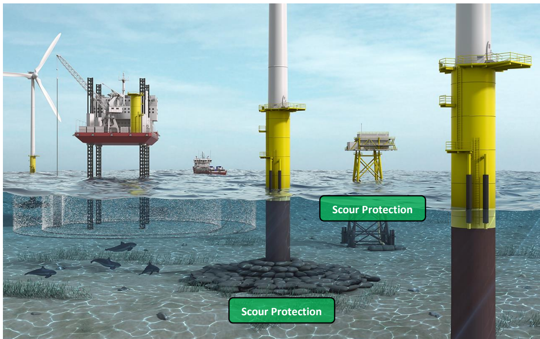
Figure 28. Scour protection example, source: [Jaeger2020].
