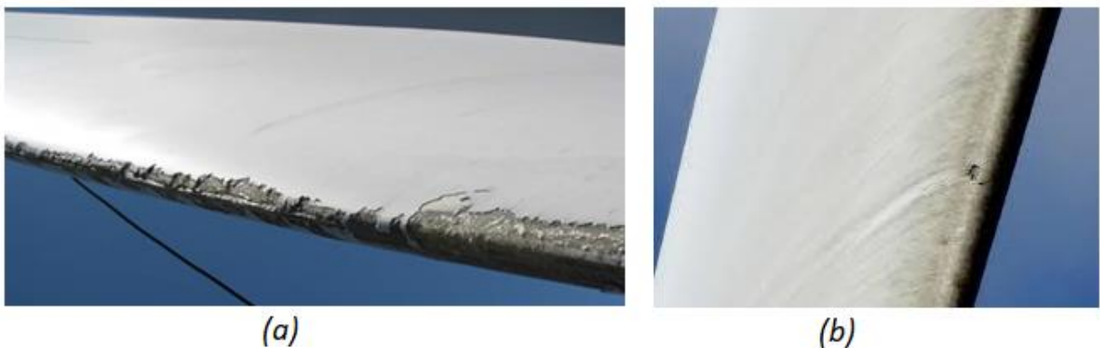
Figure 4. Blades defects: (a) leading edge erosion; (b) blade crack.
