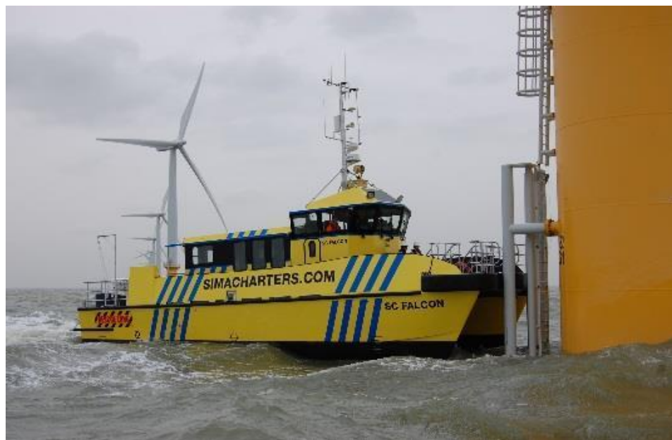
Figure 35. Transfer of staff by direct contact between vessel and windmill, source: [Ynf].
