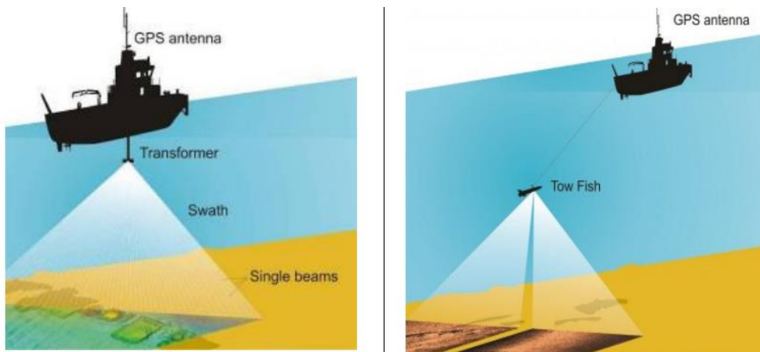
Figure 29. Survey vessel with multi-beam or side scan sonar, source: [GEO2005]
