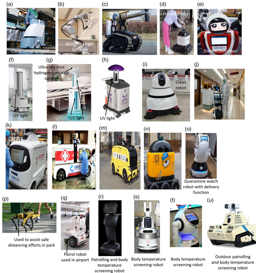
Figure 2. (a) Cleaning Robot from SoftBank Robotics. 8 (b) XDBot by Nanyang Technological University. 9 (c) Tank-style, remote-controlled disinfecting robot. 10 (d) Portable hand sanitizer robot from Zhen Rhotobics Corp. 11 (e) Aerosol Disinfection Robot from Shanghai TMI Rob Technology. 12 (f) UV-C light Disinfection Robot by UVD Robots. 13 (g) Intelligent Disinfection Robot by TMI Rob. 14 (h) UV light robot by Xenex Disinfection Services. 15 (i) Autonomous Cleaning Robot by Seoul National University Hospital. 16 (j) Pudu Technology's autonomous service delivery robot. 18 (k) JD Logistics' large self-driving delivery vehicle. 19 (l) White Rhino Auto Company's large self-driving delivery vehicle. 20 (m) Meituan's large self-driving delivery vehicle. 21 (n) ZhenRobotics' RoboPony. 22 (o) Quarantine watch robot. 23 (p) Boston Dynamics' Spot being used in Bishan-Ang Mo Kio Park, Singapore. 24 (q) Smart patrol robot being used in Guiyang Airport, China. 25 (r) Temi robots, 26 (s) AIMBOT, and (t) Cruz robots from UBTECH. 28 (u) Atris outdoor screening and patrolling robot from UBTECH. 30
