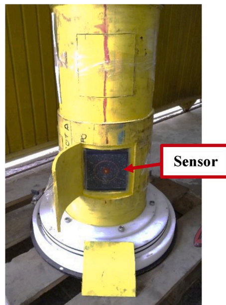
Fig. 5. Segment of the flexible pipe with openings for the insertion of sensors.
