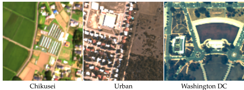
Figure 8. Reference remote sensing images with 93 spectral bands and spatial resolution of 128 \times 128 used in the experiments of Section 5.2. We display 7th, 25th and 40th bands to account for the blue, green and red channels.
