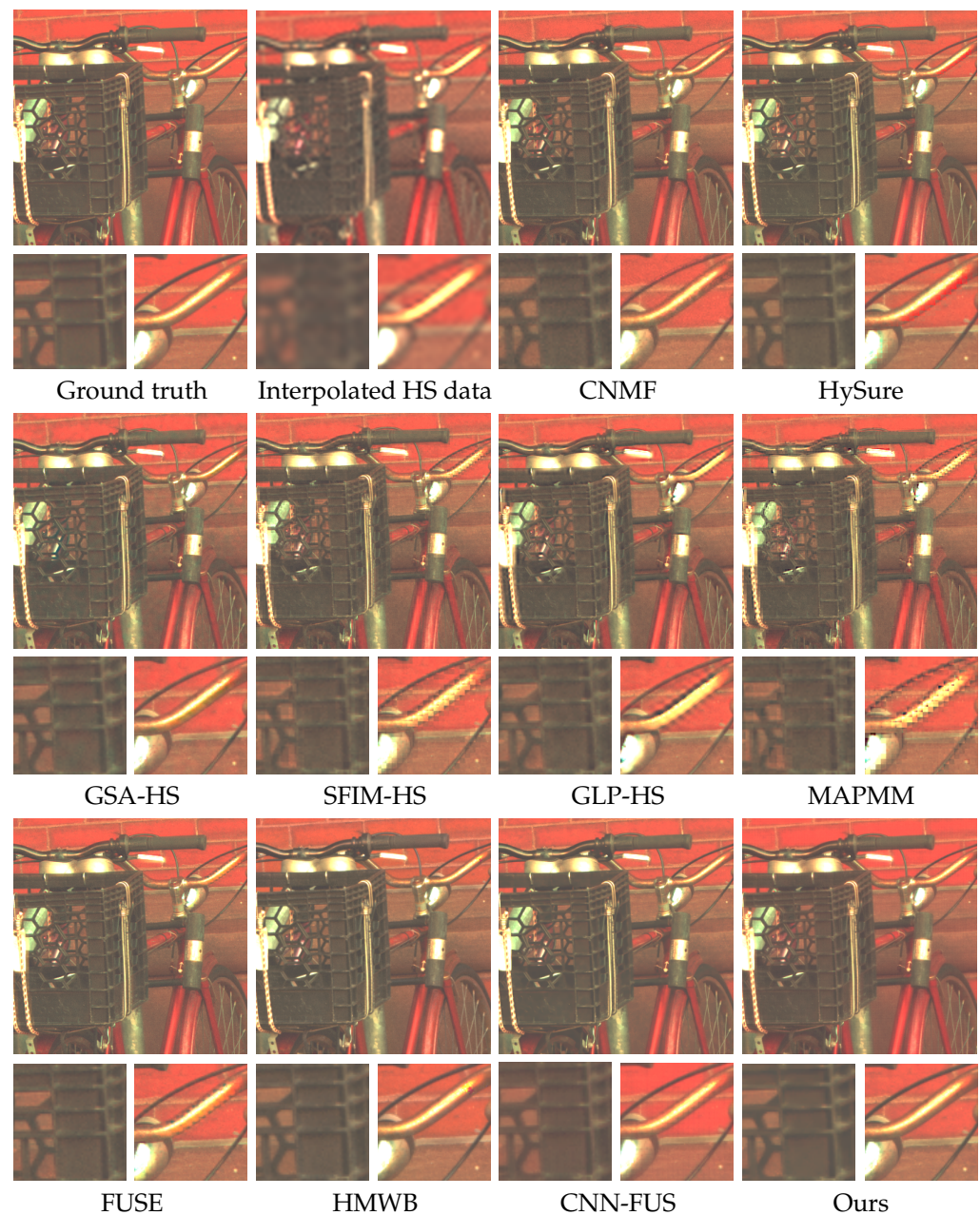
Figure 7. Visual comparison of the fusion approaches on Bicycles. All techniques except ours are affected either by noise (see the baskets) or by aliasing effects in the form of color spots and jagged edges (see the metal handlebars). The proposed fusion method successfully combines the geometry and spatial details of the MS image with the spectral information of the HS image, while removing noise and avoiding distortions due to aliasing.
