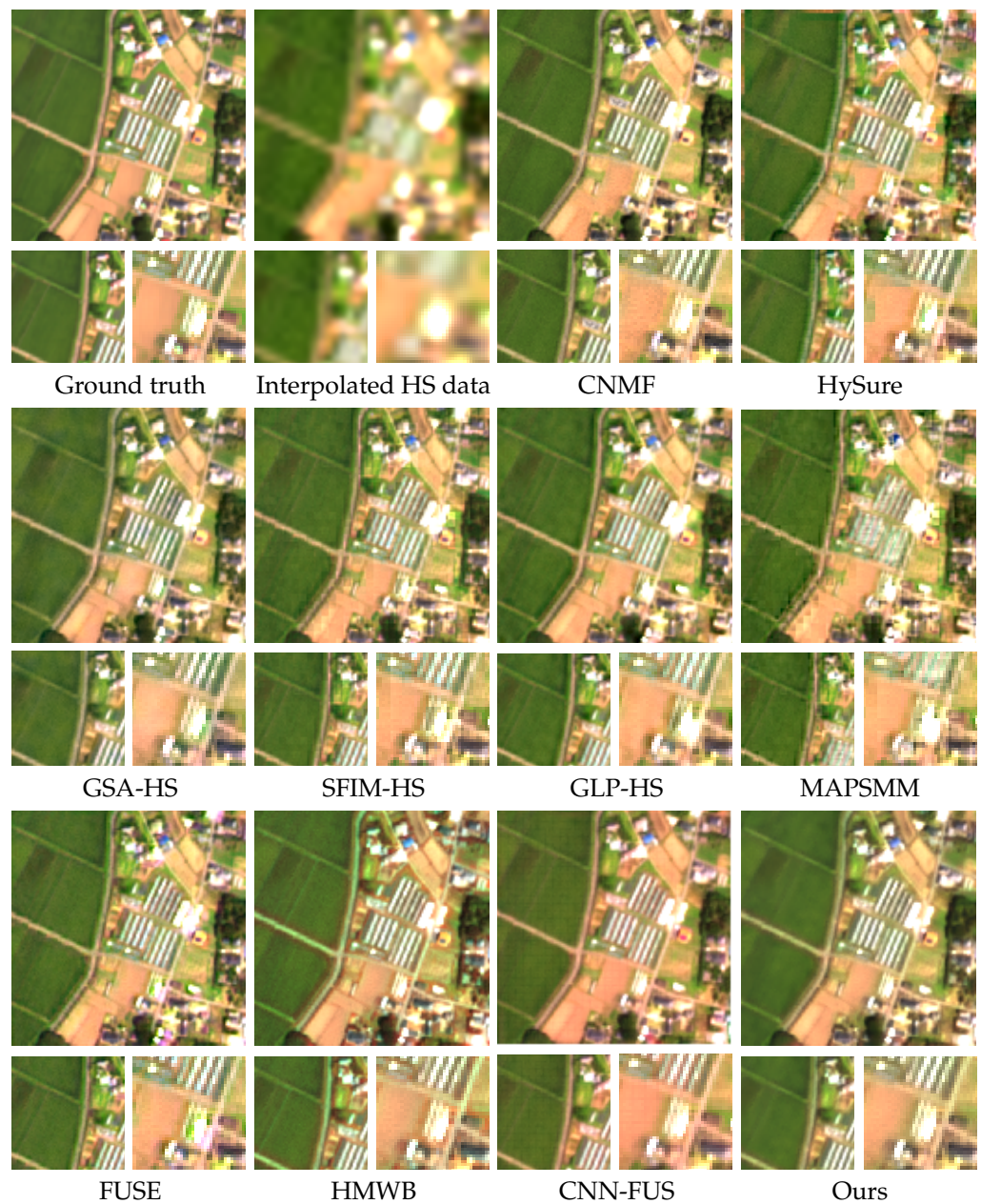
Figure 9. Visual comparison of the fusion methods on Chikusei. All state-of-the-art methods are not robust to noise, and only the proposed approach is able to remove it while preserving the spatial details of the scene. Annoying artifacts further compromise the results provided by HySure, SFIM-HS, MAPMM and FUSE. We also observe that HMWB is not able to correctly recover the spectral information from the HS data, while GLP-HS have problems at saturated areas such as light reflections on roofs. Regarding CNN-FUS, we notice the appearance of small repetitive squares especially on the green parts. Furthermore, the white building have some pink color influence which does not exist on the ground truth image.
