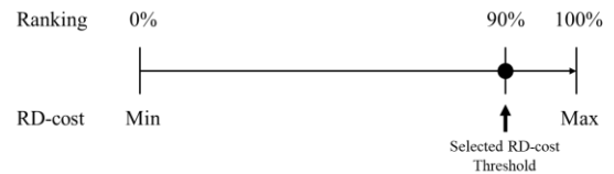
Fig. 17 Illustration of selecting the RD-cost threshold.
