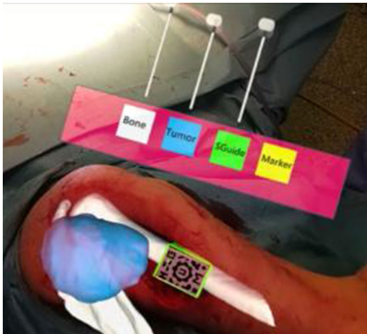
Fig. 1 HoloLens view during the surgery after the tumor resection. The virtual bone and tumor are projected overlaid on the patient in the correct position. A virtual panel allows controlling the transparency of the virtual biomodels
