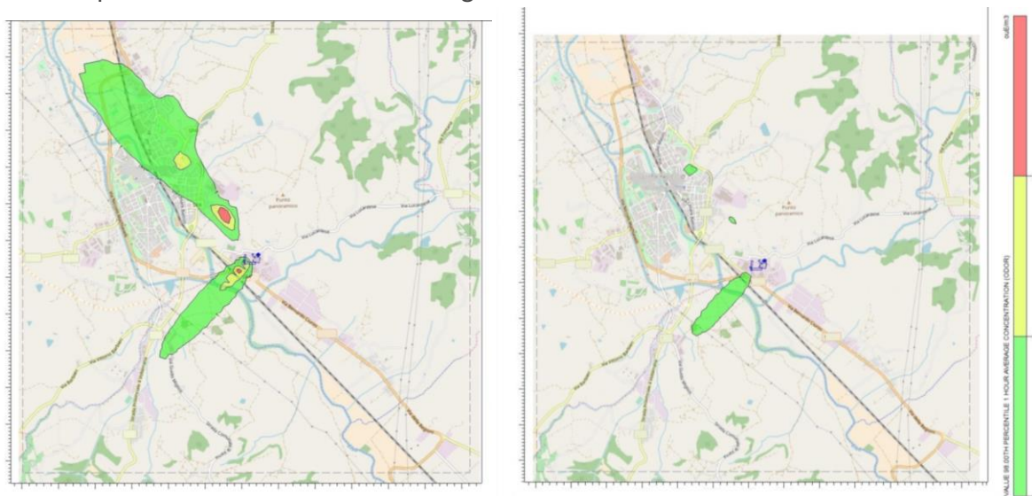
Figure 23: Comparison of the odour impact related to the emission from a stack with a height of 27 m (left) and 50 m (right)
