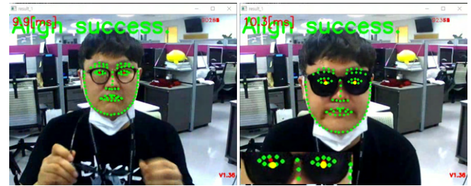
FIGURE 7. Examples of comparison of the predicted pupils from the proposed algorithm and the ground truth points on sunglasses faces. All the ground truths of eye positions were annotated as precisely as possible via comparison with the corresponding bare face images (left). Yellow points indicate the ground truth points of pupil center positions and red points indicate the predicted pupil center positions by the proposed algorithm (right).
