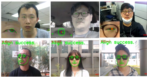
FIGURE 6. Experimental results on bare faces with 11 eye-nose landmark points with iris regression (top row), and sunglasses faces with 98 whole facial points with eye position refinement via feature map re-weighting (bottom row). For bare faces (top row), the green dot inside the pupil circle indicates the initial eye position from SDM and the red dot indicates the refined eye center position using the proposed iris regression algorithm. For sunglasses faces (bottom row), the red dots indicate the estimated pupil position and the green dots indicate the remaining facial points.
