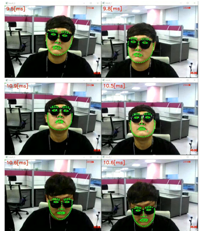
FIGURE 12. Eye-tracking results on sunglasses faces videos (640x480 stereo webcam). The left column indicates the left camera views and the right column shows the right camera views from the stereo webcam. The algorithm calculates the 3D pupil coordinates from these two pupil points from the stereo camera.
