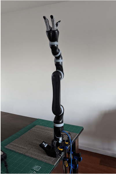
Fig. 2. The setup of the Kinova Mico 2 arm. The “candle” pose allows for the zeroing of torque sensors before operation and a safe start configuration to begin torque control. The robot is connected via ethernet connection and with small amendments to the kinova-ros package that inhibits the data published by the publisher to the minimum required for the task so as the communications with the arm is able to achieve 25Hz.
