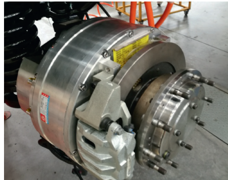
FIGURE 7: In-wheel motor assembly system.
