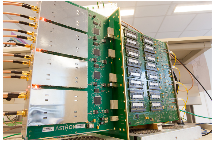
Fig. 21. The Analog to Digital conversion board (left), midplane (center), and UniBoard (right), cover removed.
