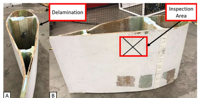
Figure 20. A- Side on view of the decommissioned wind turbine blade displaying the delamination on the interior of the blade. B- Straight on view of the exterior of the decommissioned wind turbine blade highlighting the inspection area.
