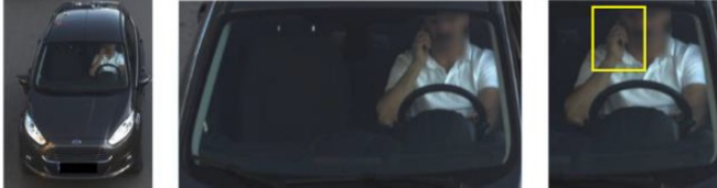
Fig. 2: The three-stage mobile usage violation detection approach of Alkan et al. [27].
