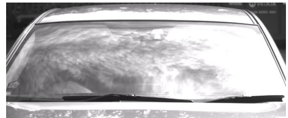
Fig. 5: Image during sunny/cloudy day without a polarising filter to show the adverse effects of windscreen reflection.
