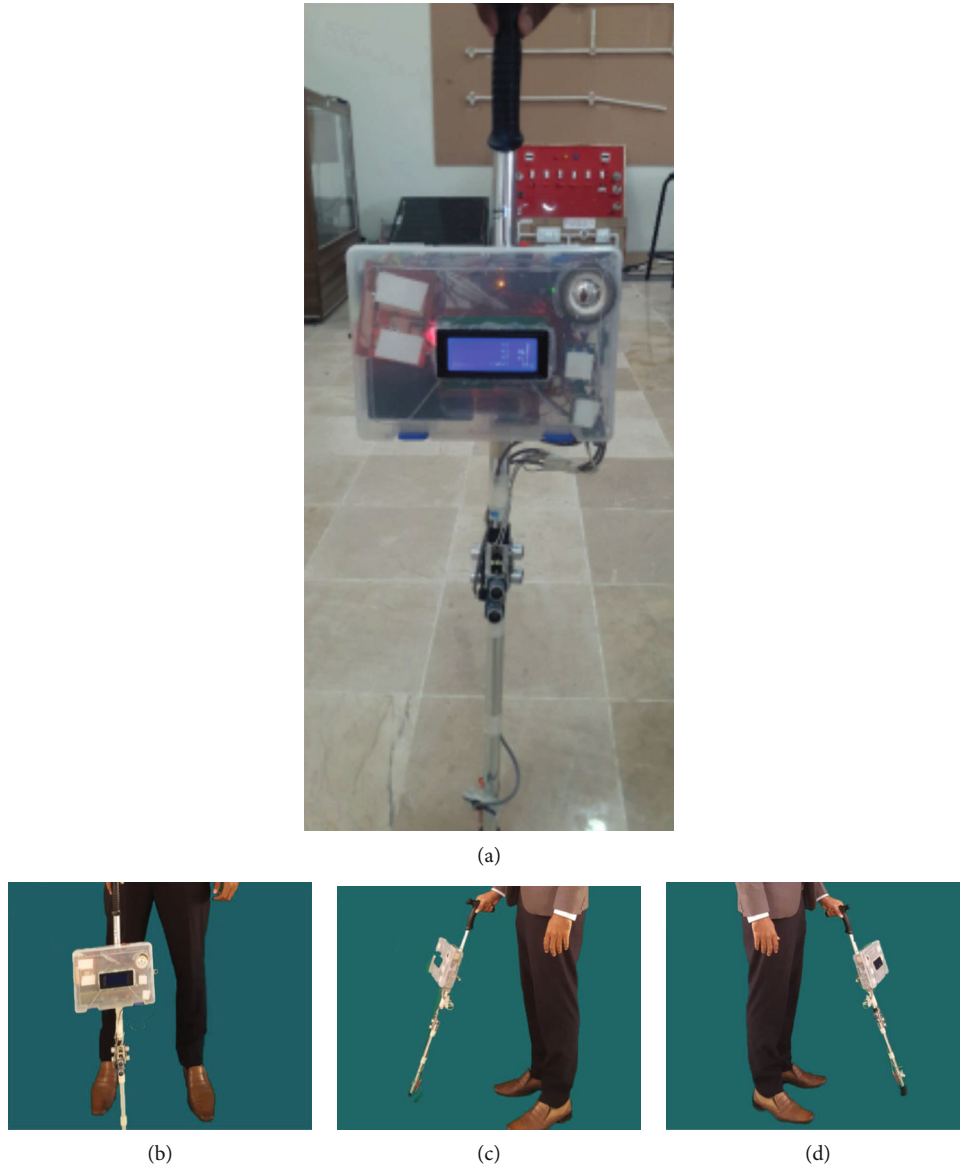
FIGURE 7: Result diagrams of the indoor area of the smart aid electronic stick to move “forward,” “turn right,” and “turn left” at object detection. (a) In the real-time simulation, the proposed system finds the path by the situation of the surface and the place of the object on it and helps decide to which direction to move. (b) In the representation, they check the obstacles if there is any and then change their path which is dictated by speaker voice. (c) When an object comes in front of an obstacle avoidance sensor, the first set dictates a command to turn left while the other remaining dictations are neglected. (d) When motion is in front of the second obstacle sensor, only the part of the second set of the visually impaired person dictates a command to turn right, and all the other positions are neglected.
