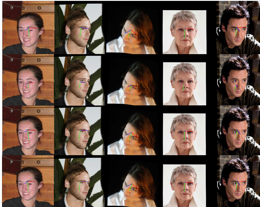
FIGURE 9. Pose estimation on the AFLW2000 dataset. From top to bottom, the GroundTruth, results of Hopenet, results of FSA-Net and our results.
