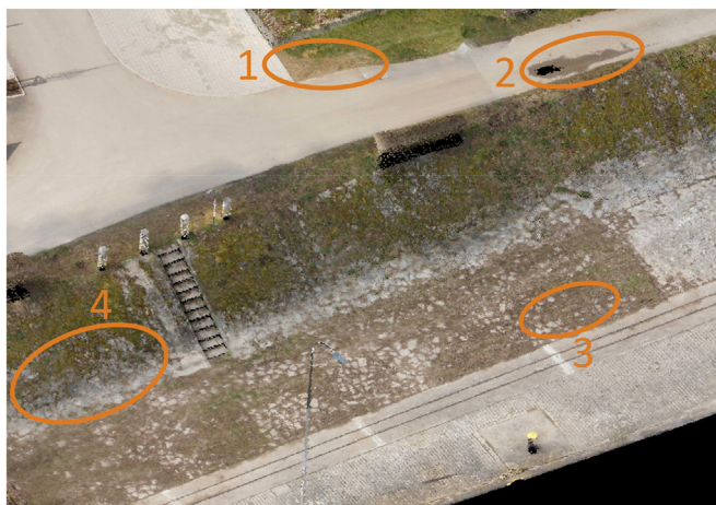
Fig. 9. Regions of distinct classes in H3D(PC) with similar radiometric properties. Issues in automated semantic segmentation based on colors can arise due to small parts of other class affiliation (1), misleading colors caused by wetness such as puddles (2) and human created structures that have been overgrown and eroded over time (3 & 4).
