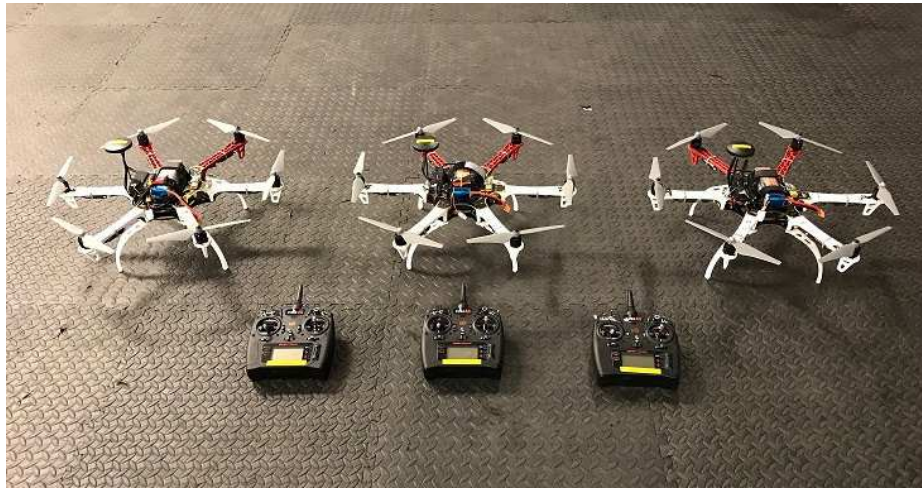
Figure 7.2: Cooperative multi-UAV system for aerial grasping in outdoor environments
