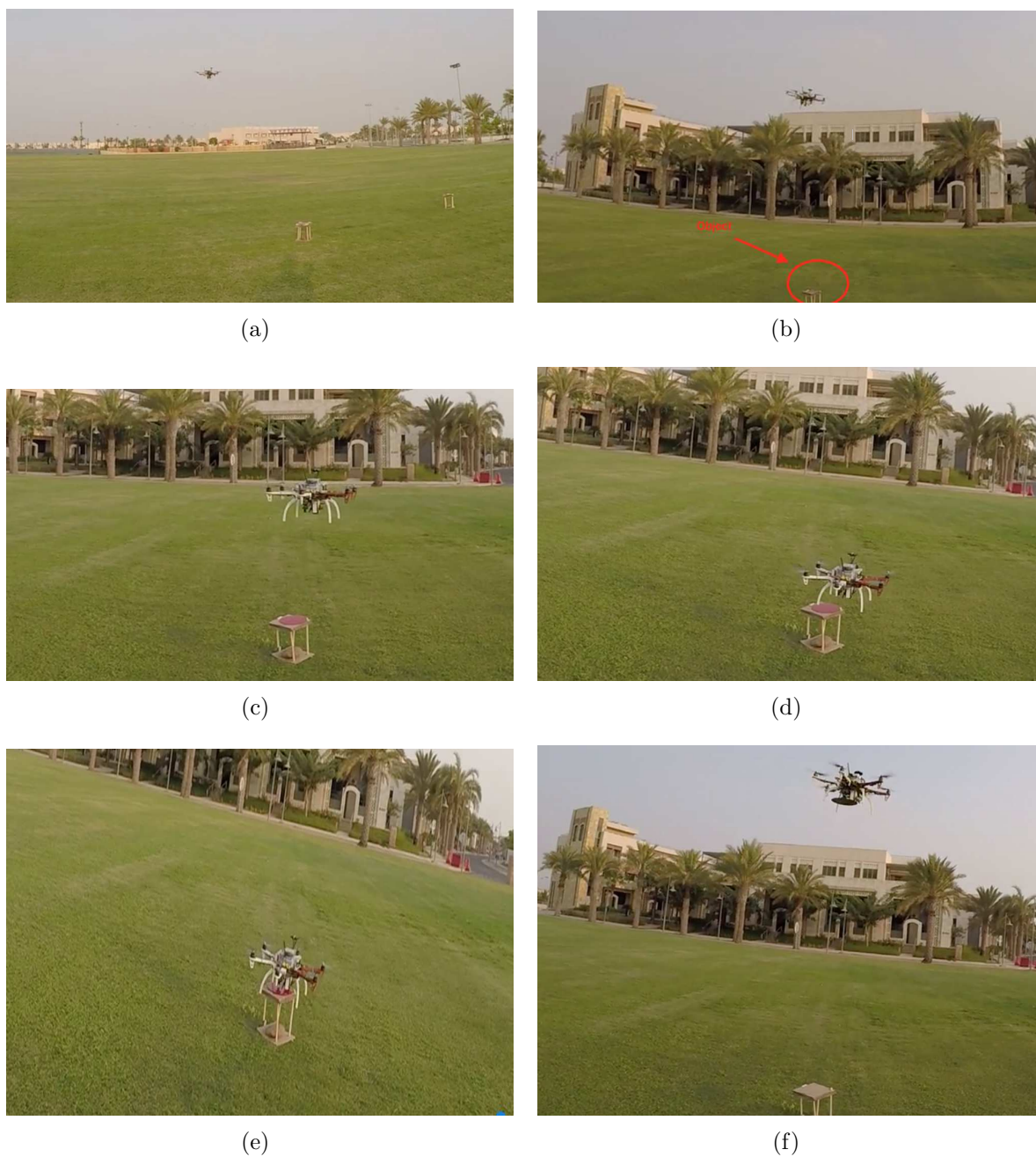
Figure 7.7: Single drone testing; (a) a snapshot of the drone in the search phase, (b) a snapshot of the drone after an object is found and selected, (c) a snapshot of the drone after an object is found and selected, (d) a snapshot of the drone while aligning over the object to prepare for picking, (e) a snapshot of the drone while picking the object, and (f) a snapshot of the drone after picking the object, going to the drop phase
