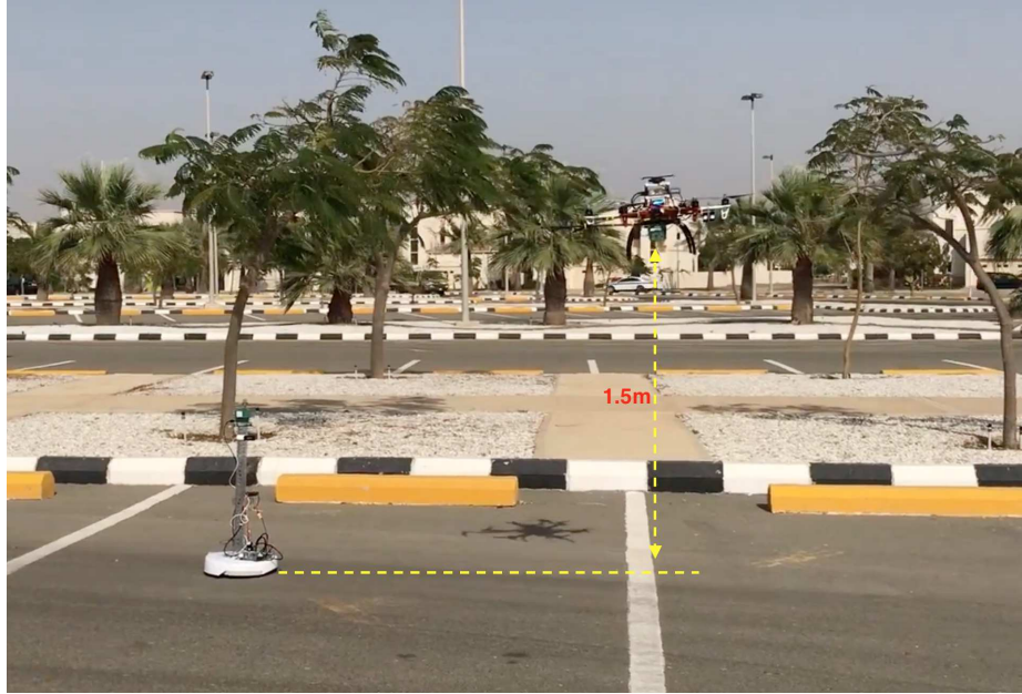
Figure 7.19: A snapshot of an outdoor trial with the ground robot moving with 0.2m/s forward velocity and the tracking drone at altitude 1.5m.
