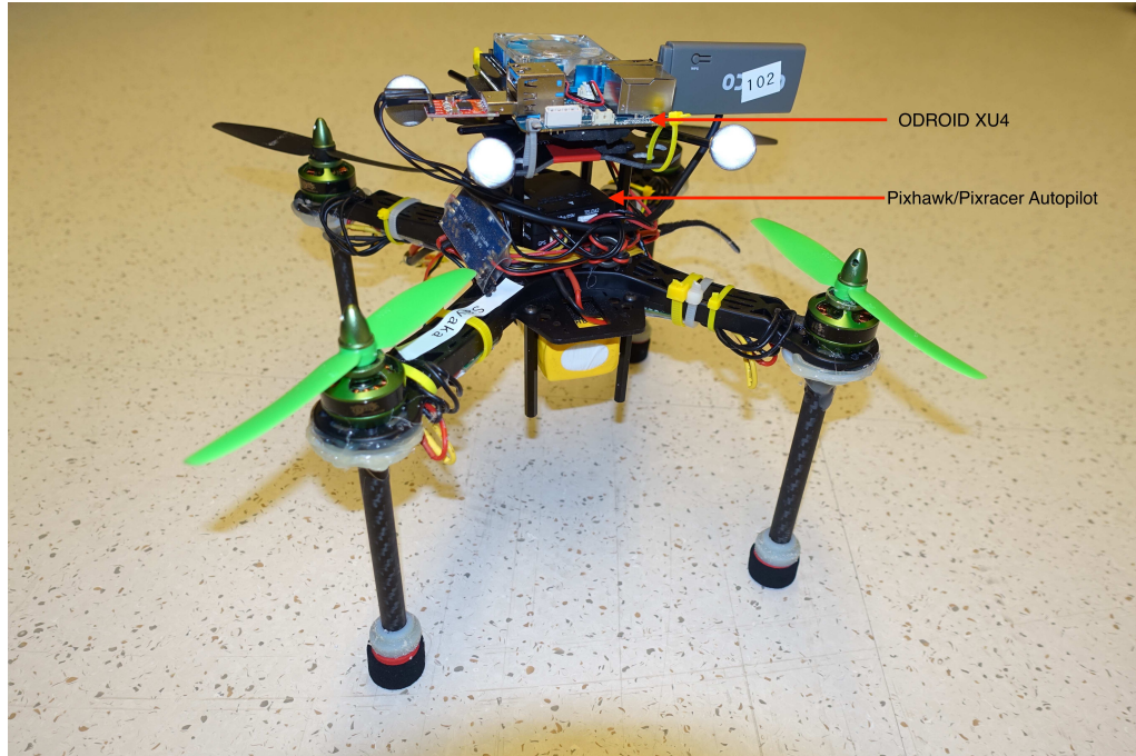
Figure 6.14: Quadrotor setup. The propulsion system composed of 2300Kv motors with 5-inch propellers and 20A speed controllers. The power is provided through a 3S LiPo battery
