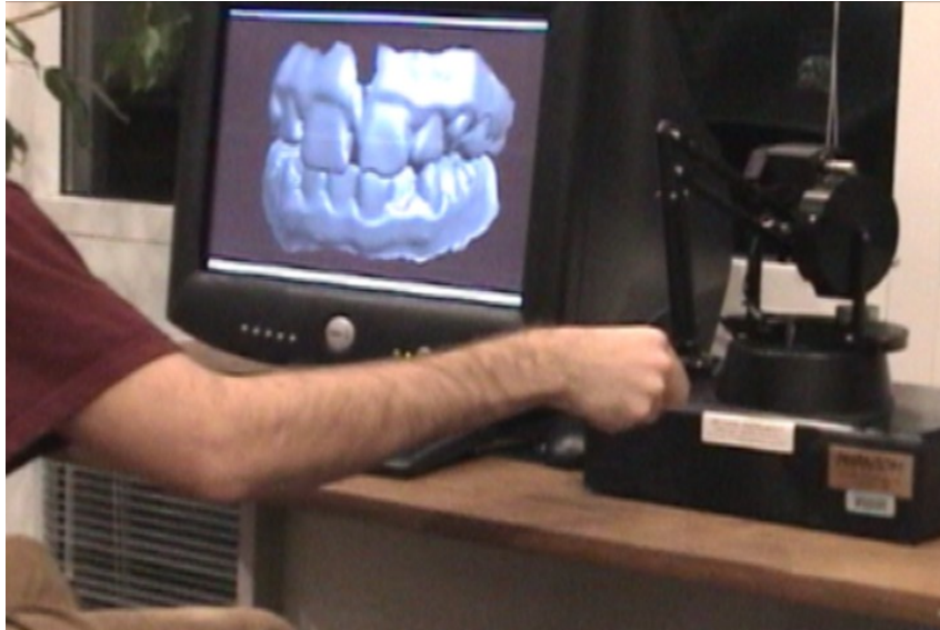
Figure 45: Example of Haptic Rendering. A person manipulates a virtual jaw using a haptic device (shown on the right of the image), and the interaction between jaws is displayed both visually and haptically.
