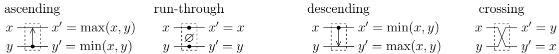
Fig. 5.14. Set of comparator elements including the computational ascending \uparrow and descending \downarrow comparators, as well as the direct run-through and crossing elements which are used for a symbolic representation of the networks.
