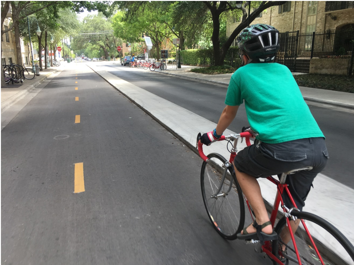
Figure 9: Two-way Protected Bike Lane on Rio Grande Street, Austin, TX (photo G. Griffin, June 10, 2018).
