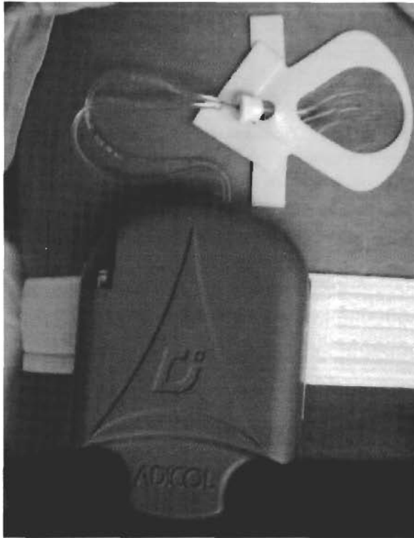
An integrated glucose sensor and insulin pump developed under the ADICOL project. The sensor is implanted under the skin to continuously measure and display the blood sugar concentration.
