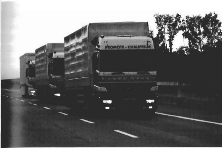
Demonstration of an automatically-steered three-vehicle convoy (Photo: CHAUFFEUR2 project)
