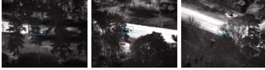
FIGURE 1: Some examples of VIVID-infrared images carefully selected, in which 40% area of the vehicles is occluded by the complex background.
