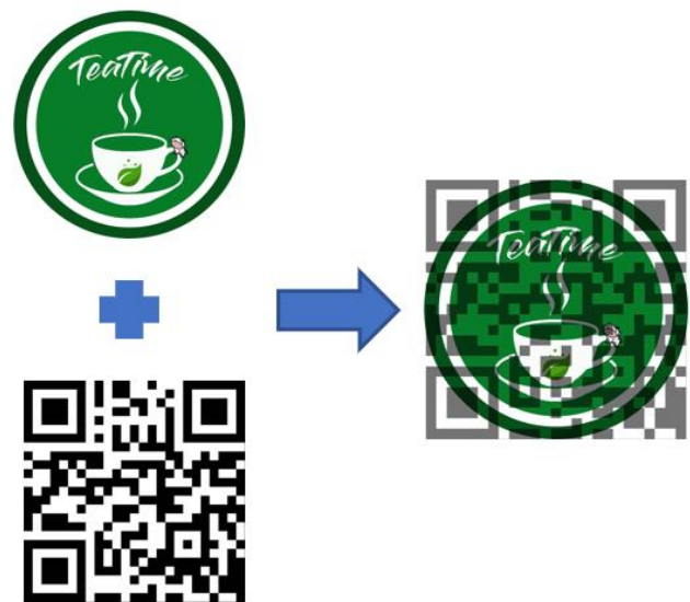
Fig. 2. The example of hybrid marker from color community brand image in opacity layer mode.
