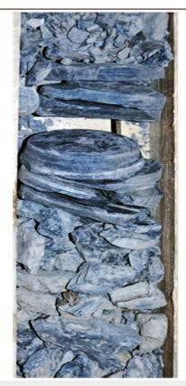
Fig.4. Photo of a core sample: mudstone broken into pieces from the 4982–4990 m interval,
