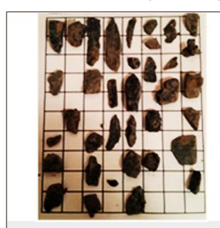
Fig.3. Photo of cuttings fallen from a depth of 3522 m, Well 75 (Scale: 2 cm in a cellule)
