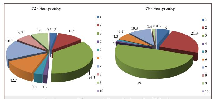
Fig.7. Percentage of time spent during production casing drilling for: 1 – BHA make up; 2 – hoisting operations; 3 – drilling; 4 – connection; 5 – gauging; 6 – other operations; 7 – reaming; 8 – gauging and reaming; 9 – hole cleaning; 10 – tool recovery using different methods
