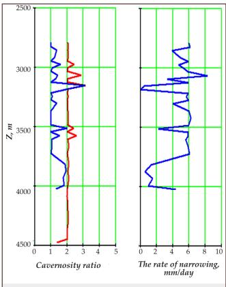
Fig.2. Caliper logs (--- of March 6, 2019 and --- of March 25, 2019) and the average rate of hole closure, Well 72- Semyrenky
