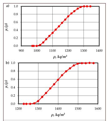
Fig.6. Membership functions for mud weight for problem prevention at depths:
