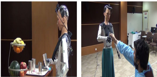
Fig. 5: Images of the Telepresence and Teleoperated robot "Asha". Left side: Grasping water glass from table. Right side: Handing the water glass to a human.
