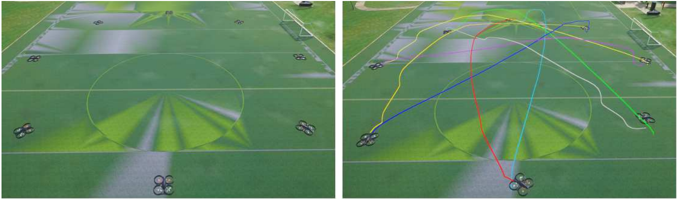
Fig. 1. left: The Airsim simulator used in this paper. right: UAVs trajectories in the Circle scenario using our learned policy.
