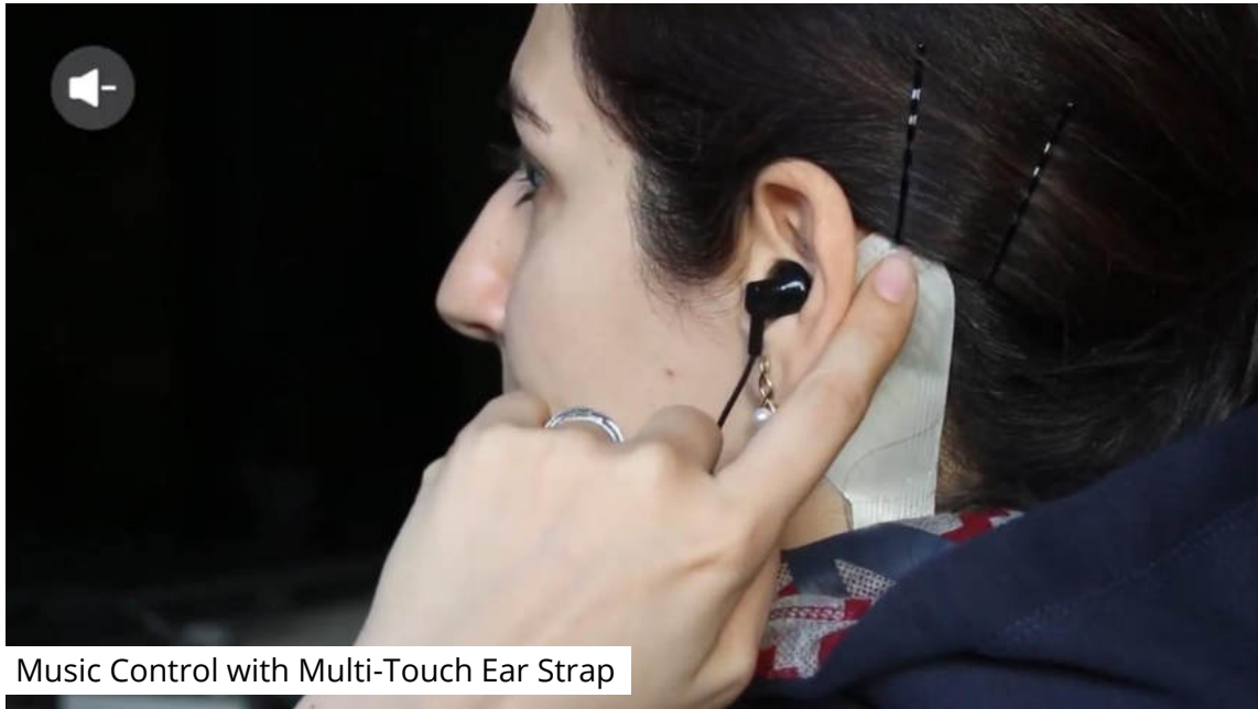
Figure 46: Multi-Touch Skin deployed on the ear to support quick access to music control. In this specific scenario, the user can perform a simple vertical and horizontal swipes to control volume or to switch music tracks.
