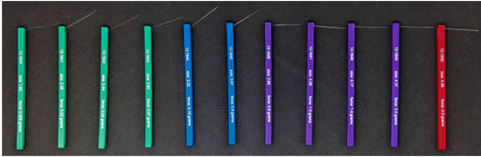
Figure 17: Von-Frey Filaments used in the Tactile Sensitivity experiment. Each of the filaments has a force profile starting with the lowest force of 0.008 grams to 4.0 grams.
