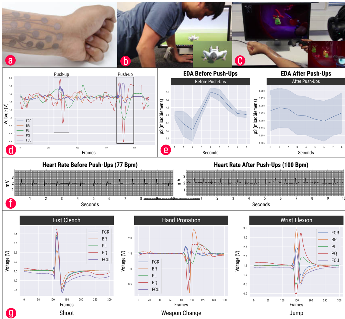
Figure 75: Example applications. (a) Ultra-thin temporary tattoo with compact sensor layout generated by the optimizer and fabricated with an off-the-shelf desktop ink-jet printer. (b) Augmented reality exercising application: a virtual character performs push-up motion when the user performs a push-up. (c) A virtual reality game in which EMG-sensed gestures are used for controlling the virtual character in a first-person shooter game. (d) Raw signals of the EMG signals when performing a push-up exercise. (e) Increase in the skin conductivity levels before and after the push-ups. The shaded region represents the standard deviation. (f) Difference in the heart rate before and after performing the push-ups. (g) Raw EMG signals of the five muscles for each of the gestures used in the virtual reality game.
