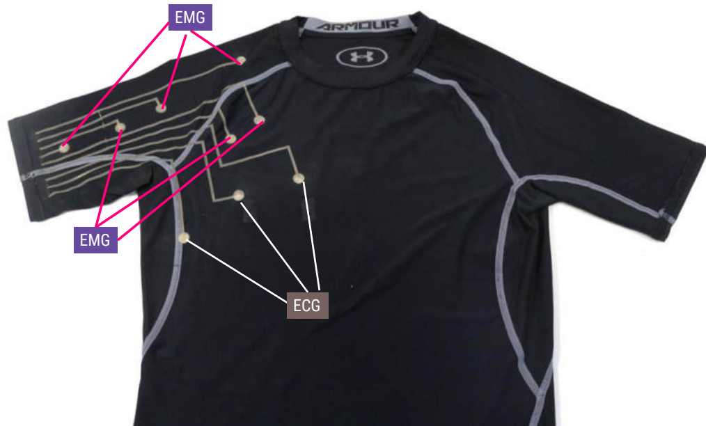
Figure 57: A fitness tracking vest with electrodes for EMG and ECG sensing.
