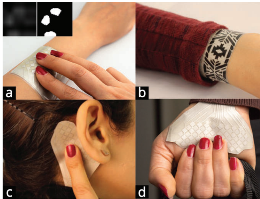
Figure 32: The thin and flexible multi-touch sensor can be customized in size and shape to fit various locations on the body: a) multi-touch input on the forearm for remote communication (inset shows capacitive image); b) multi-touch-enabled bracelet with an art-layer for aesthetic customization; c) input behind the ear; d) input on the palm with busy hands.
