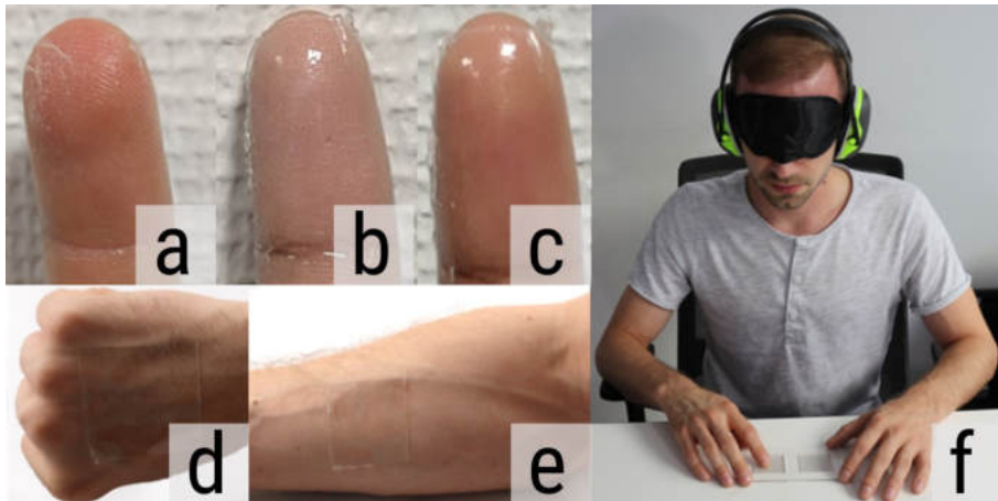
Figure 16: Three patch conditions with varying levels of flexural rigidity: (a) Patch with low rigidity level ( \sim 1.7 \times 10^{-9} ), (b) medium rigidity ( \sim 1.3 \times 10^{-7} ), (c) high rigidity ( \sim 1.7 \times 10^{-5} ). Patches were applied on (a) the Fingertip , (d) Hand and (e) Forearm . (f) Participant performing roughness-discrimination task.
