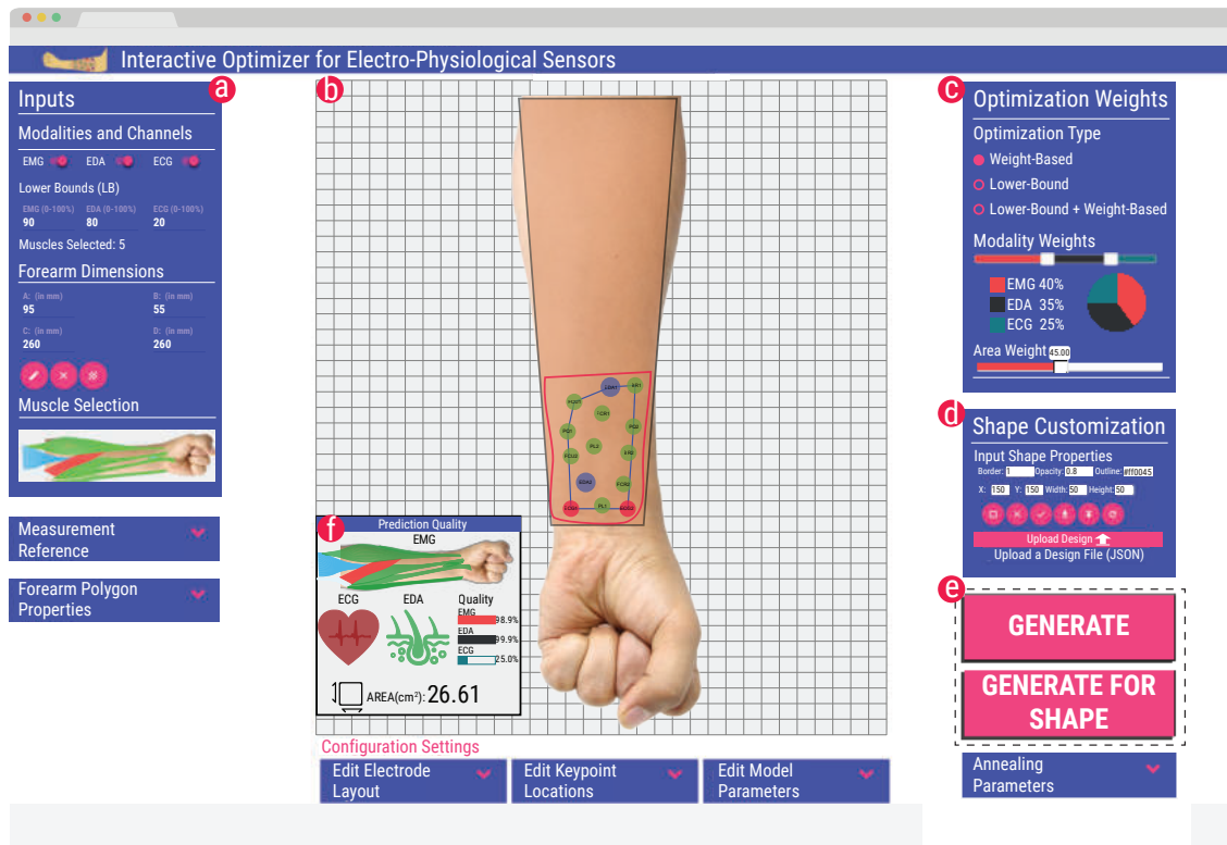
Figure 63: Screenshot of the graphical design tool for interactively generating and inspecting optimized results. (a) Input panel for selecting the modalities and muscles, setting forearm dimensions, and setting the lower bounds. (b) The canvas area where the generated designs are visualized. Designs can be fine-tuned by drawing a desired location and shape or dragging individual electrodes. (c) Panel for choosing the optimization type, weights for each of the modalities, and overall sensor area. (d) Shape customization panel for fine-tuning the properties related to the sensor shape. Additionally, this panel also allows for uploading existing designs and exporting the current designs. (e) Buttons for one-click automatic generation of the layout. The result is displayed in real-time in the canvas area. (f) Panel visualizing quality metrics for the generated layout. Advanced functionality for use by experts can be accessed through drop-down panels. This includes functions for adjusting and editing the electrodes in the generated solution, adjusting the internal parameters of the model, tweaking the optimization parameters, and adjusting the appearance of the forearm polygon. The workflow for using the tool is shown in Supplementary Video 1.
