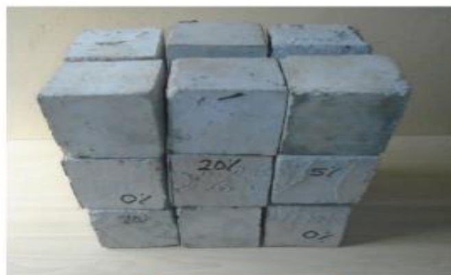
Fig. 2: Rubberized Masonry Concrete Cubes for Dynamic Mechanical Test
