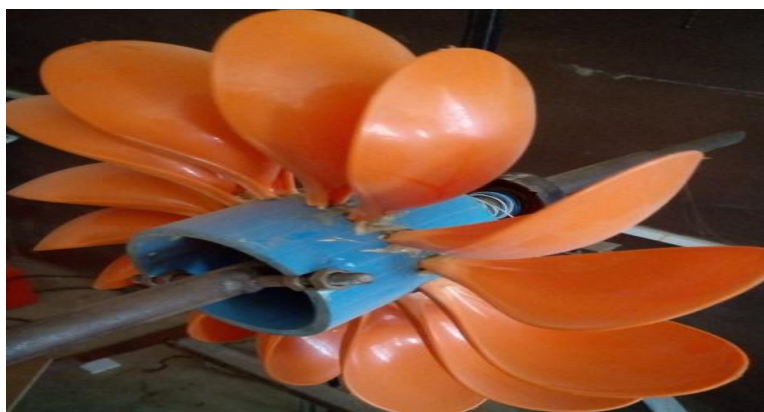
Figure 4: Locally fabricated Turbine blades used in the hydro power set up
