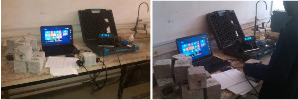
Fig. 3: Ultrasonic Pulse Velocity Test of Reference and Rubberized Concrete
