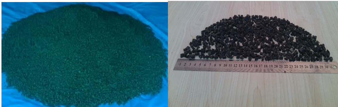
Fig. 3: Crumb-Rubber partially used for the Production of Masonry Hollow Concrete Blocks.
