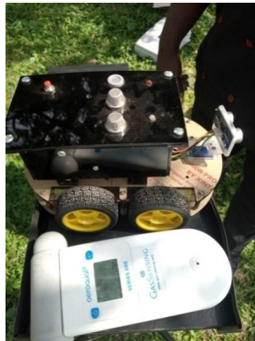
Figure 8. The developed system with Aeroqual series 300 during data capture
