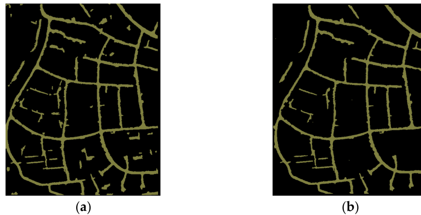
Figure 18. Road point extraction results after two-step post-processing. (a) Smoothing the road points of Figure 17d with graph-cut; (b) Clustered non-road points removal from Figure 18a based on CTINs.
