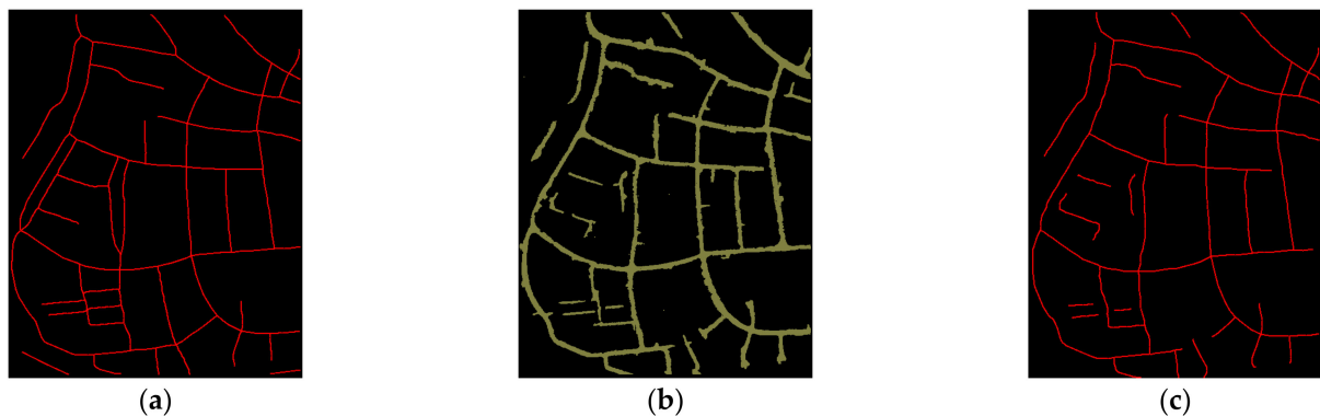
Figure 19. Centerline extraction result. (a) True centerlines obtained from Figure 17a by hand editing; (b) Duplicate of Figure 18b for comparison; (c) Centerlines extracted from Figure 19b by the proposed framework.
