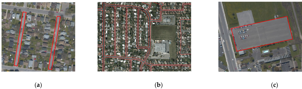
Figure 12. Illustration of the shape difference between a road and a parking lot. (a) Local Road; (b) Road Network; (c) Parking Lot.
