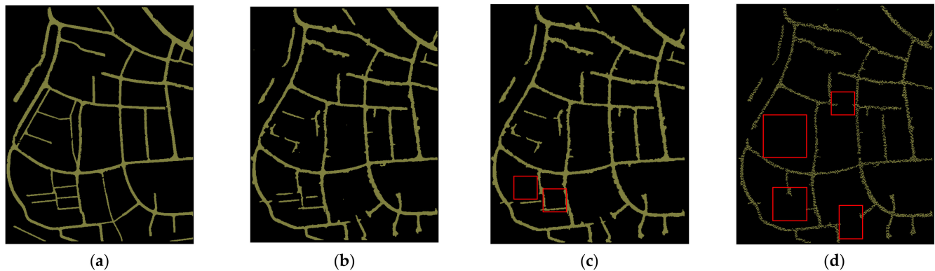
Figure 20. Road points extracted under different point densities. (a) True road points. (b) Density = 4 points/m 2 . (c) Density = 1.0 points/m 2 . (d) Density = 0.25 points/m 2 .
