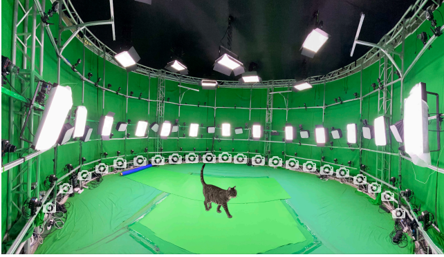
Fig. 7. Setup of our animal motion capture system. The system consists of 12 Vicon cameras and 22 Z-CAM cinema cameras surrounding the animal.
