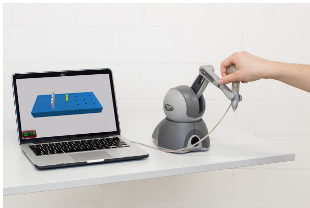
Figure 6: The Virtual Peg Insertion Test (VPIT) is a technology-aided assessment platform consisting of a haptic end-effector, a grasping force sensing handle, and a virtual reality environment. It allows recording of kinematic and kinetic data about sensorimotor impairments in arm and hand during a functional task.
