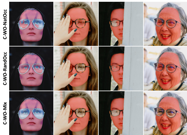
Figure 10. The visual results on transparent/translucent occluders of SegFormer [35] trained on C-WO-NatOcc, C-WO-RandOcc and C-WO-Mix. Models trained on C-WO-NatOcc and C-WO-RandOcc failed to detect transparent glasses as occlusion accurately. In contrast, the model on C-WO-Mix can detect transparent glasses as occlusions, proving that RandOcc is complementary to NatOcc to detect transparent/translucent objects.
