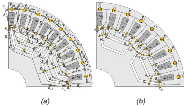
FIGURE 7. The on-load MEC model of the IPMSM: (a) q -axis model and (b) d -axis model.
