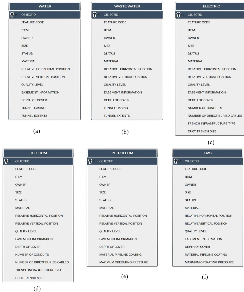
FIGURE 2. Attributes for the six types of utilities which include a) water, b) waste water, c) electric, d) telecom, e) petroleum, f) gas.
