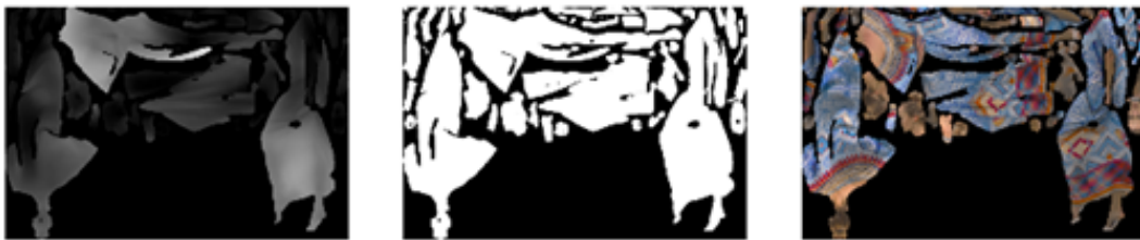
Fig. III-3. Example of geometry (left), occupancy map (center), and attribute (e.g., texture) (right) images.
