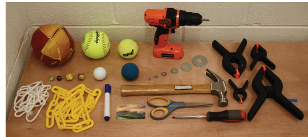
Fig. 9. The YCB object set, used entirely in the grasping capability evaluation and partially in the in-hand manipulation evaluation of the gripper.
