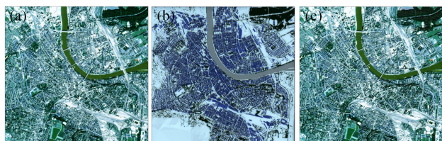
Fig. 8. (a) PlanetScope image in the Basel area. (b) DART image simulated with constant SS per urban component. (c) The DART image after the calibration procedure. All images are RGB color composites.
