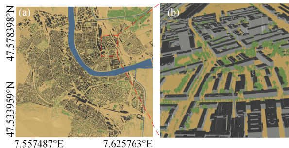
Fig. 7. Basel 3D digital surface model (DSM). (a) Top view. (b) Side view of the red square in (a). Buildings (roofs: dark, walls: light grey), trees (green), river (blue), and ground (yellow).
