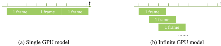
Figure 3.4: Two computation models considered in our evaluation. Each block represents an algorithm running on a device and its length indicates its runtime.
