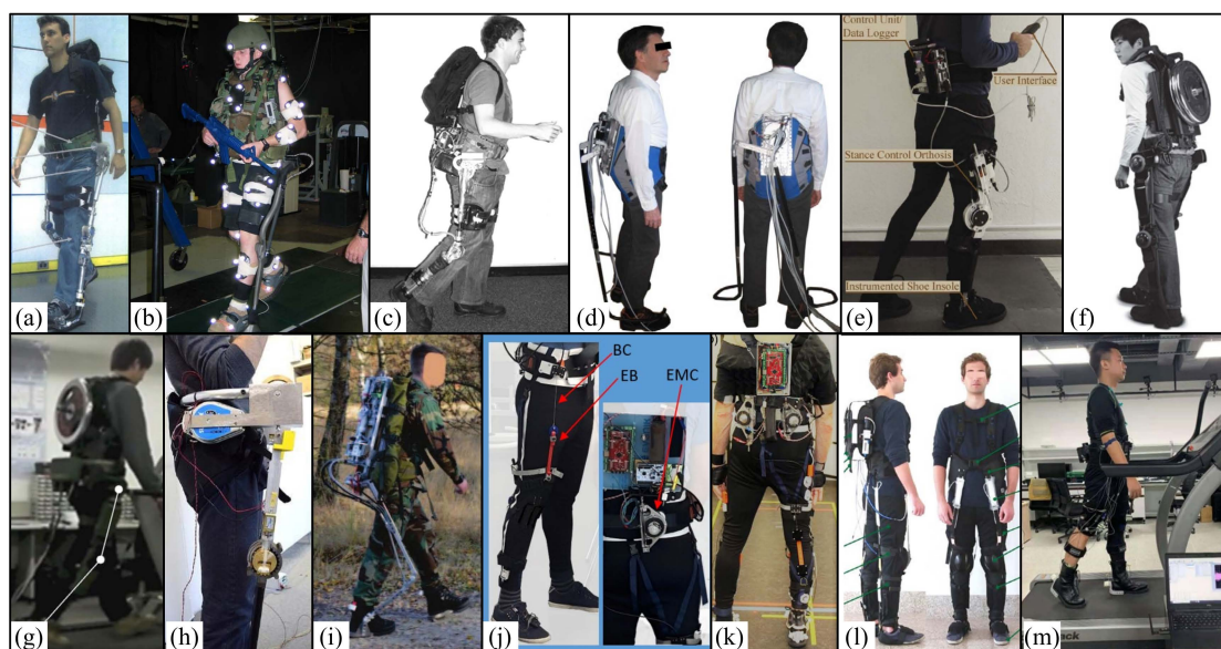
Figure 7. Multi-joint lower limb assisted exoskeletons. (a) MIT, QPPLEALCW [110]. (b) US Army Natick soldier Center, LBELCAD [112]. (c) MIT, QPLELCA [3]. (d) University of Montpellier, Moonwalker [113]. (e) Yale University, QPCSKAFO [114]. (f) Hanyang University, HEXAR, Seoul, Korea [116]. (g) Korea Atomic Energy Research Institute, UEEWLCA [118]. (h) Tokyo University of agricultural technology, QPLLEPBWS [119]. (i) Netherlands applied scientific research organization, Exobuddy [120]. (j) Italian Institute of Technology, SWDLLA [121]. (k) Italian Institute of Technology, SALLE [122]. (l) Italian Institute of Technology, SALLE [123]. (m) Shenzhen Institute of Advanced Technology, Chinese Academy of Sciences [124].
