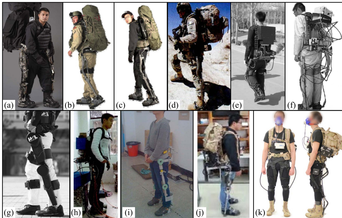
Figure 3. Multi-joint powered lower limb assisted exoskeleton. (a) University of California, BLEEX [8]. (b) ExoHIKE [48]. (c) ExoClimber [48]. (d) Lockheed Martin, HULC [43]. (e) Naval Academy of Aeronautical Engineering, the third-generation prototypes [50]. (f) East China University of Technology, ELEBOT [52]. (g) University of Tsukuba, HAL-5 [59]. (h) Southwest Jiaotong University, 2012 [63]. (i) Harbin Institute of Technology, 2013 [61]. (j) Beijing University of technology [63]. (k) Harvard University, MJSE [65].
