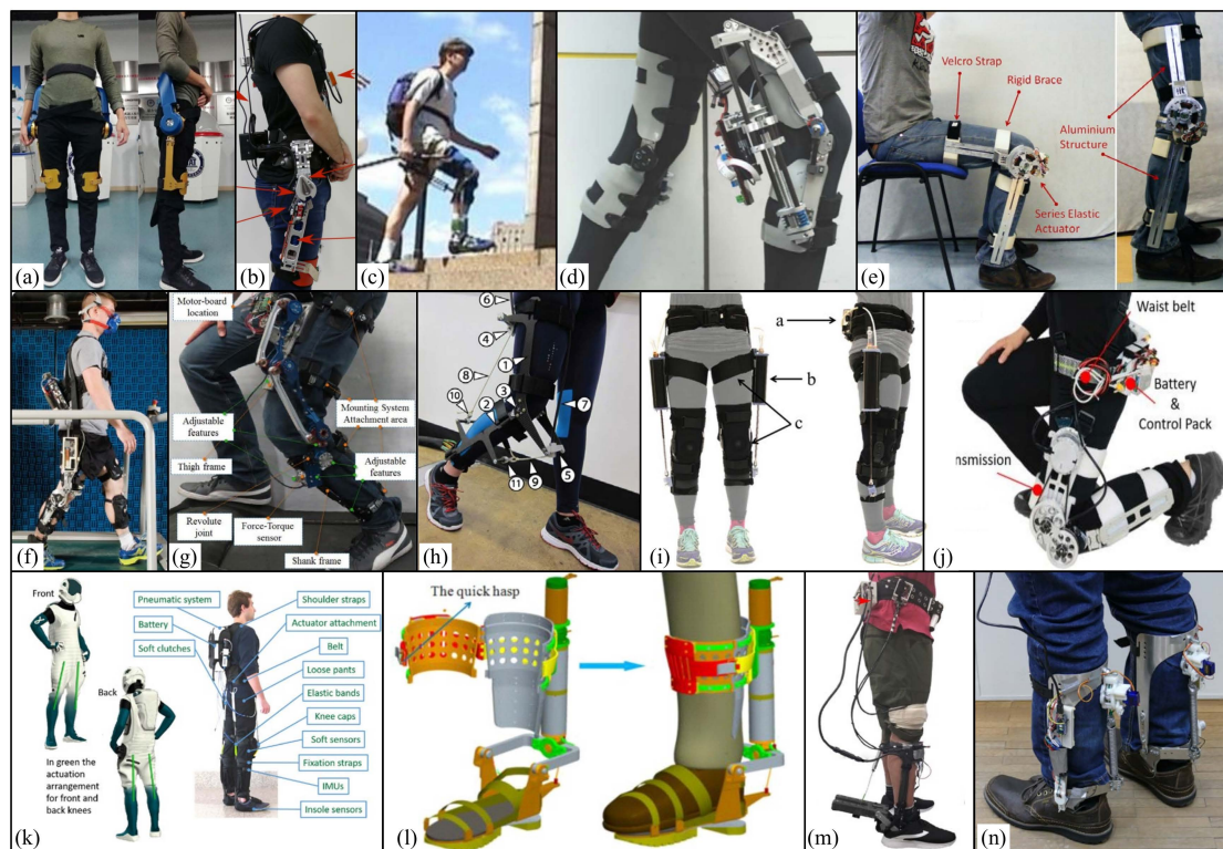
Figure 8. Single-joint quasi passive lower limb exoskeletons. (a) Chinese Academy of Science (CAS) [125]. (b) Slovenia, CQPSE [126]. (c) University of Michigan, RoboKnee [127]. (d) Carlton University, QPKEAR [128]. (e) Italian Institute of Technology, ACCKE [130]. (f) Yale University, QPKEGE [132]. (g) Italian Institute of Technology, iT-Knee [133]. (h) Carnegie Mellon University, LTTCKE [134]. (i) Harvard University, QPKEADD [135]. (j) City University of New York, LBKE [5]. (k) Italian Institute of Technology, QPRESA [136]. (l) Harbin Institute of Technology, QPAFWRO [137]. (m) University of Texas, SATQPAE [138]. (n) Ljubljana, Slovenia, CAAE [139].
