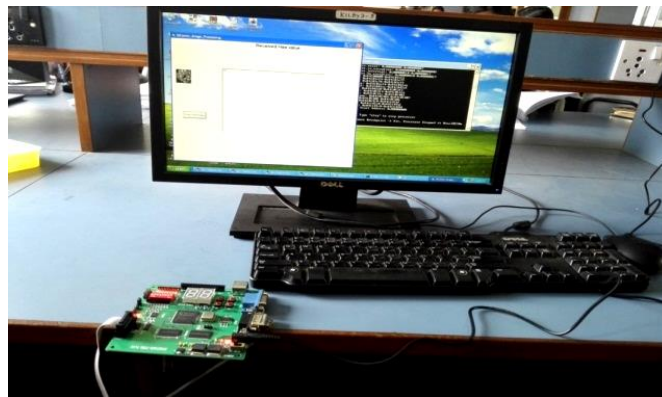
Figure 9. Hardware implementation of FPGA using embedded Microblaze core processor
