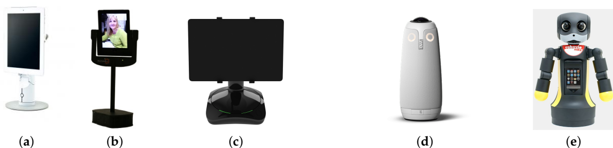
Figure 4. Unmovable robotic telepresence (RP) systems: (a) Kubi, (b) TableTop TeleMe, (c) SelfieBot, (d) Meeting Owl Pro, and (e) Robovie mR2.
