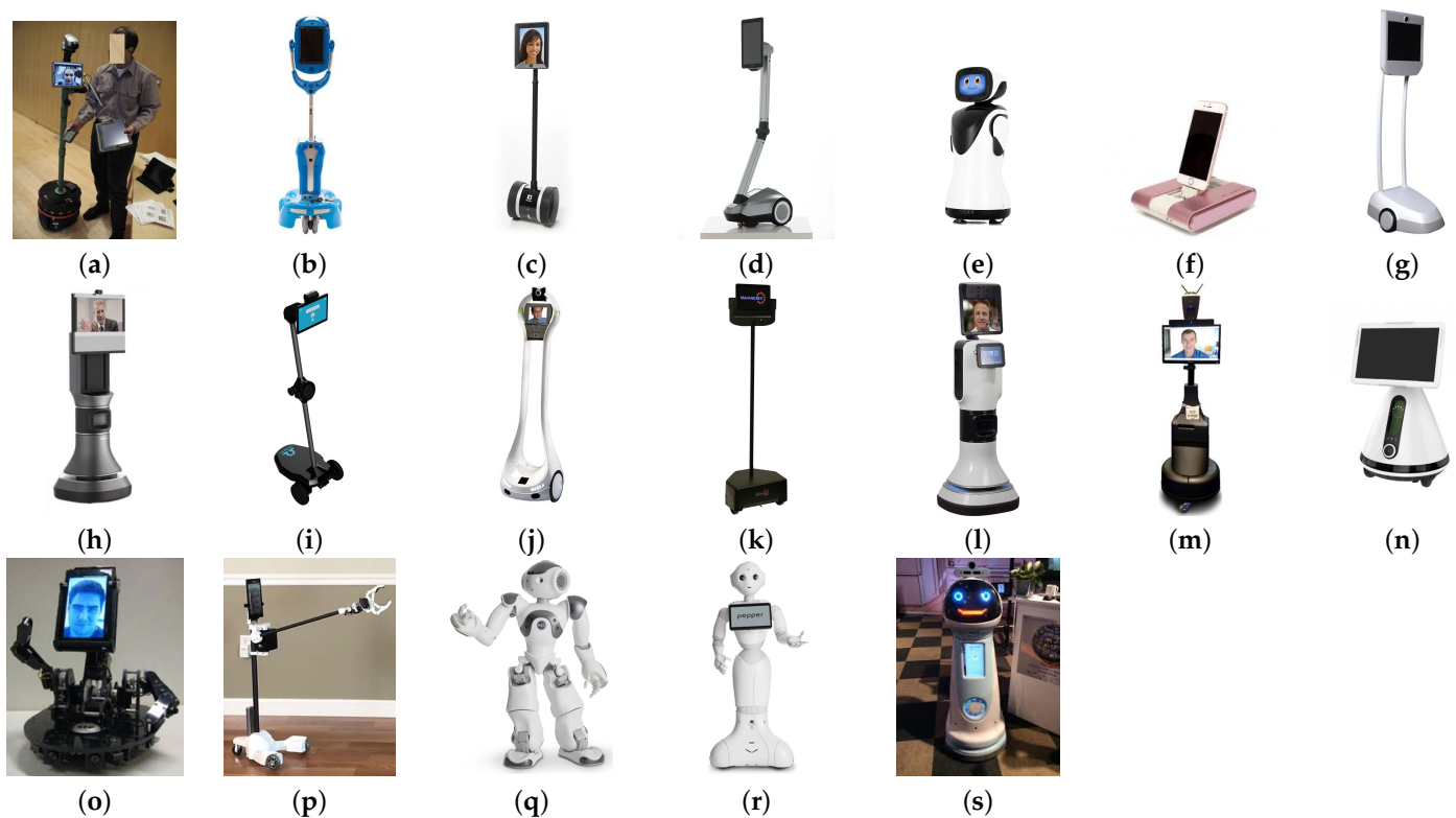
Figure 3. Mobile robotic telepresence (MRP) systems: (a) PRoP, (b) Giraff, (c) Double 2, 3, (d) PadBot 2, (e) PadBot 3, (f) PadBot T1, (g) Beam Pro, (h) Ava 500, (i) Ohmni SuperCam, (j) VGo, (k) TeleMe, (l) RP-Vita, (m) Teleporter, (n) FURo-i, (o) MeBot, (p) Oritbot2, (q) Nao, (r) Pepper, and (s) GrowMeUp.
