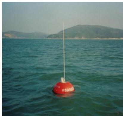
**Figure 4.** SBF series coastal telemetering wave gauge.
