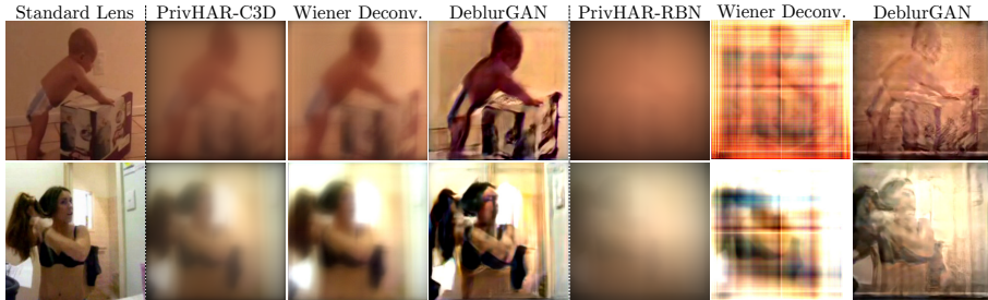
Fig. 5. Deconvolution of private images acquired with our optimized lens using C3D and Rubiksnet (RBN) backbones in PrivHAR. The images acquired with our lens are robust to deconvolution, and DeblurGAN cannot recover people’s identities.
