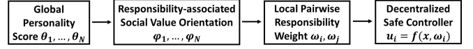
Fig. 3: Proposed framework. We propose the concept of Responsibility-associated Social Value Orientation (R-SVO) to measure the relative difference in agent personalities. Local Pairwise Responsibility Weight uses the information from (R-SVO) and is applied as a weight in the CBF-based decentralized safe controller to solve the responsibility allocation problem in multi-agent collision avoidance.
